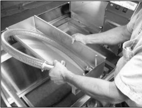
33. Remove the glaze reservoir and hose.
